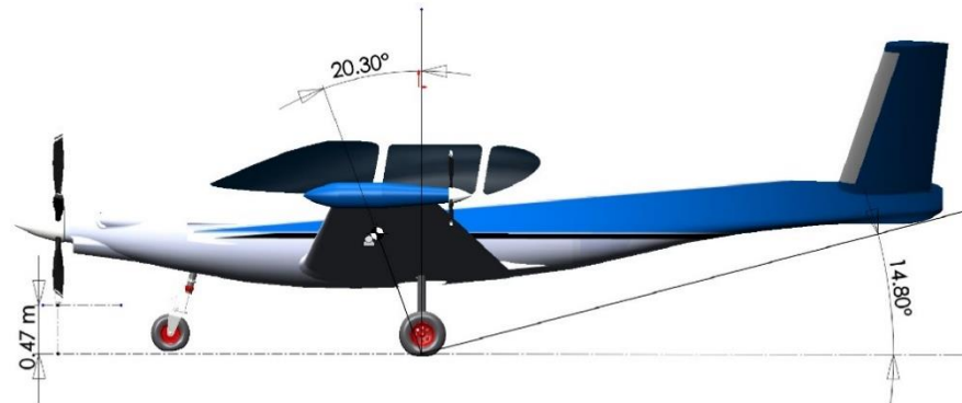
50. Positioning of the Main Landing Gear
